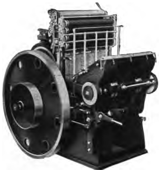
Fig. 1. Platen Press with Automatic Safety Stop. (Pat.)
